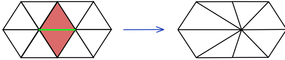
Figure 4.8: Single edge collapse iteration. Collapsing the green edge removes the red faces and results in the mesh on the right.
